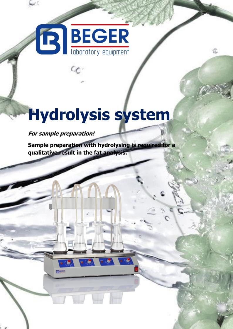
Hydrolysis systems of the BEGER Company are used for sample preparation in the determination of fat content in a foodstuff and feed. Sample preparation with hydrolysing is required for a qualitative result in the fat analysis. HYDRO apparatus provides a
